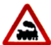
Railway level crossing without gate or barrier
